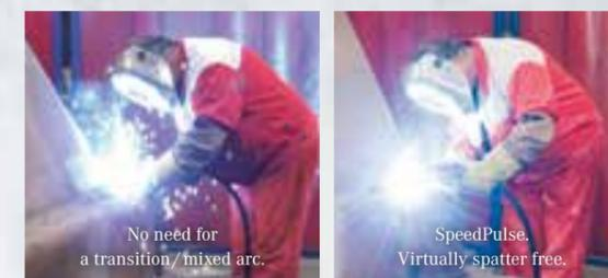
A pointed wire end, allowing the arc energy to be focused directly into the weld throughout the entire current range. As in the case with standard MIG-MAG welding filler wire spools no longer need to be changed depending on material thickness to be welded. No unnecessary changes of wire spools. For example you can weld 1.0 mm metal sheets with 1.2 mm filler wire and weld smoothly and without interruption – up to the maximum current range. SpeedPulse also makes the complete process colder. This
