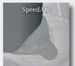
With SpeedArc, penetration into the parent material is visibly better compared to ordinary MIG-MAG units.
