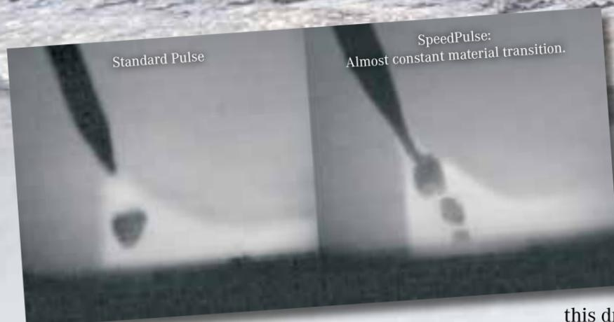
this drop, thus permitting a controlled, almost constant metal flow into the weld pool.
