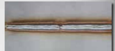
I-seam, CrNi t = 0.8 mm, root gap = 0.8 mm
